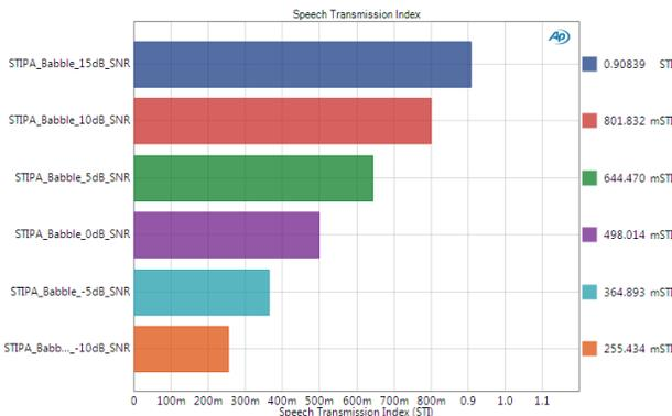
STIPA signal mixed with noise at various signal-to-noise ratios.
