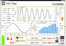
While performing tests, all necessary values like test voltage, PD-level, frequency, dissipation factor as well as a PD-pattern are shown in a single screen.
