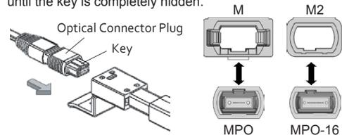
3. Insert the main body straight in to the optical connector plug. When you hear the click sound, the cleaning is completed. Stop pushing and remove straight out.
