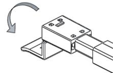
2. Align the attachment and the optical connector plug. Insert the plug straight into the attachment and push in until the key is completely hidden.
