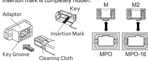
3. Push the main body straight into the Adaptor. When you hear the click sound, the cleaning is completed. Stop pushing and pull straight out.
