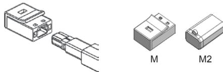
2. Align the adaptor and the guide key. Insert the guide straight into the adaptor until the cleaning cloth or the insertion mark is completely hidden.
