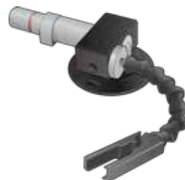
1902084 4559790 X2 VACUUM HOLDER Sensor holder with suction cup for various placements. Attached with a flexible arm and compatible with parts from X2 flexi stand.
