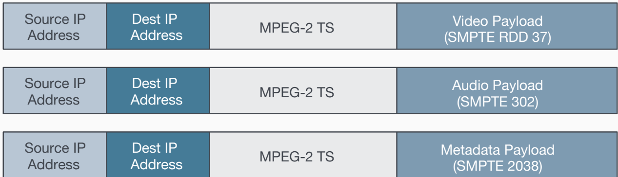
FIGURE 6. ASPEN IP Packet Formats. Dedicated IP Flows Carry Video, Audio and Metadata Essence over TS.
