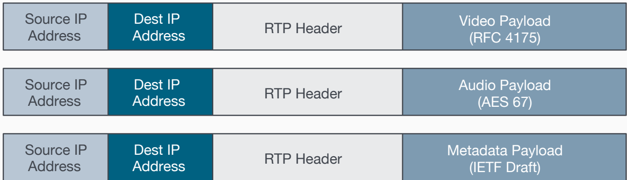
FIGURE 5. VSF TR-03 IP Packet Formats. Dedicated IP Flows Carry Video, Audio and Metadata Essence.
