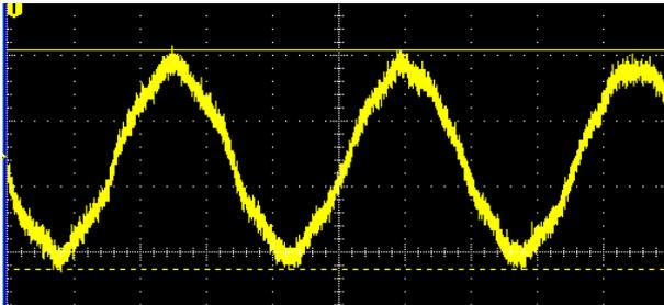
A second oscilloscope capture of the same switching amplifier output shown in Figure 4, after the application of the AUX-0025 filter. The switching carrier has been greatly reduced.
