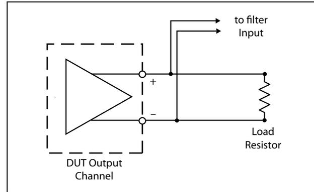
**Connection detail, DUT output, AUX filter input and load resistor.**
