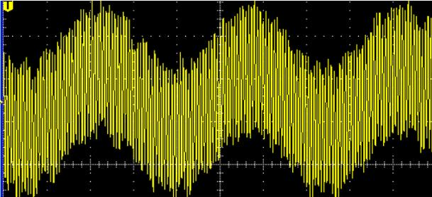
An oscilloscope capture of a switching amplifier output signal. The high-frequency, high-level switching carrier is shown riding the lower-frequency audio.
