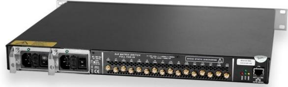
This Tx matrix distributes 8 Broadband signals to 8 antennas in the frequency range 20...3000 MHz without any blocking.
