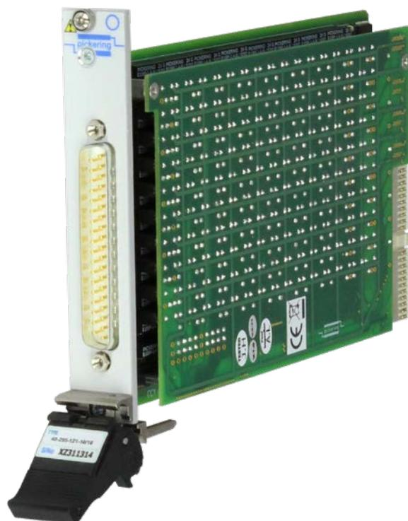
The 40-295 is a programmable resistor module with up to 18 resistor chains with 8-bit resolution in a single PXI module. The module can also be supplied in 12, 16 or 24-bit resolution versions for applications requiring finer resolution, greater resistance range or higher channel count. The module is ideal for simulating sensors for control and management systems, or verifying system response in design verification or manufacturing test.
