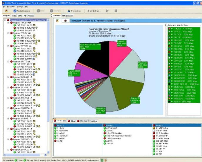
The analyzer is specifically designed to enable quick location and identification of problems within a Transport Stream using a minimum number of mouse clicks. By quickly identifying the problem areas, the TSCA software helps you save time during the development and test of equipment, networks, and services.
