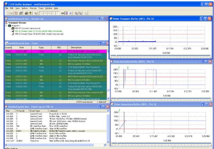
There are two types of buffer model. The one to use by the receiver is signaled within the Elementary Stream itself. The T-STD method is based upon the DTS values within the PES header and can be used for any contained CODEC type. Additionally, certain video CODECs such as MPEG-2 and H.264/AVC may contain buffer parameters within the ES itself. The Buffer Analyzer verifies conformance of a stream to the T-STD model. Verification of the H.264/AVC HRD method is covered by the MTS4EA product.
