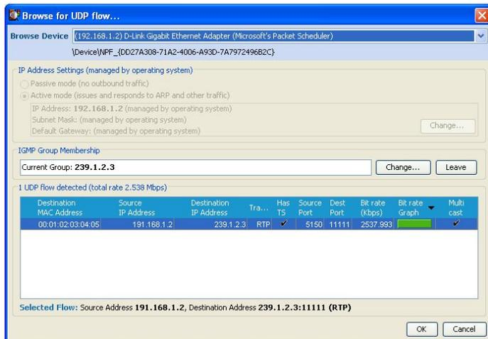
UDP sessions carrying MPEG TS traffic are indicated and may be selected for analysis and recording. Transport Stream packets are time stamped as they are received from any Network Interface Card, allowing PCR measurements and graphing to be supported. In addition, a display of the mean IP Packet Interarrival Time (PIT) histogram is available.
