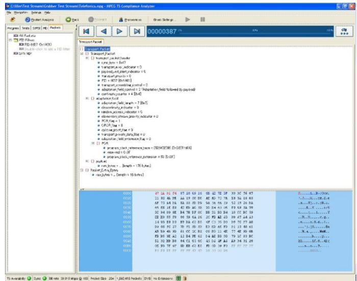
When you select a specific PID, MIP, or IP, session-only packets carrying that particular PID, MIP, or session are displayed. For Ethernet Packets, the RTP/UDP header information is displayed in both real and deferred time and can be used to display packet header information and payload.
