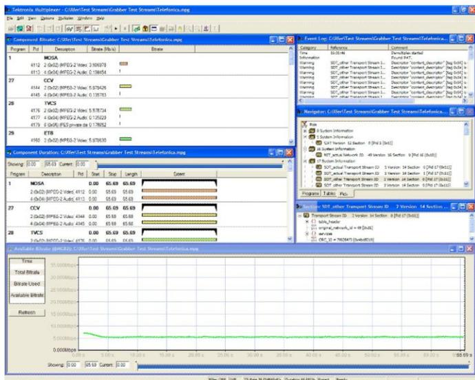
Use the Multiplexer/Remultiplexer/Demultiplexer application to create multi program Transport Streams with custom SI/PSI/PSIP information for DVB (including Annex A string support), ATSC, ISDB, and MPEG compliant Transport Streams. A new ISDB-T Single Segment mode is added in version 3.1.
