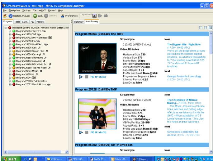
In addition to displaying a video thumbnail, the video format parameters from within ES headers are also displayed and can be checked for consistency with Transport Stream layer signaling of video parameters. This cross-check enables the operator to verify that the format of the content in the stream matches the format that they have signaled. An inconsistency could cause the STB to be unable to decode video and the viewers to lose their pictures.
