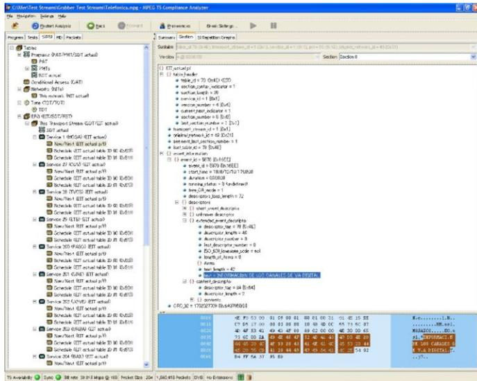
Tables and their data source are displayed. This shows the data bytes (in both hexadecimal number format and ASCII character format), for the selected table, version, and section. Tables and subtables are easily analyzed and directly traceable to packet data.
