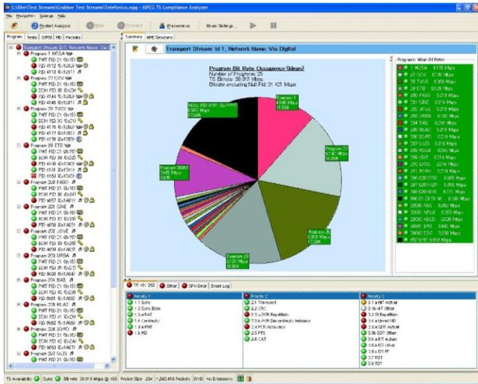
The MTS4SAV3 Transport Stream and IP Video Analyzer is a new class of analysis tool, the world's first compressed digital video debugger/analyzer that includes Tektronix CaptureVu™ technology, a capability that captures and analyzes system events in real time to debug the intermittent and complex problems that traditional analyzers miss.
