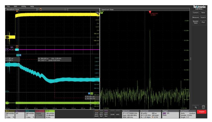
FIGURE 14. We are triggering on the SPI bus command that tells the VCO what frequency to tune to. In this case, it's 2.4 GHz. Using Spectrum Time, we were able to scroll through the acquisition and see when the RF output stabilized at 2.4 GHz. Then, using cursors, we can measure from the trigger event to Spectrum Time's location and see that it took 304 μs for the output to achieve the desired frequency.
