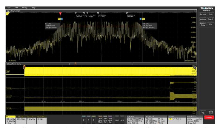
FIGURE 10. It's very easy to see what's going on with this spread spectrum clock by looking at the Magnitude and Frequency vs. Time waveforms. The Magnitude vs. Time trace shows the signal turning on at the trigger point at a very low level and the Frequency vs. Time trace shows the signal staying at a single frequency for the first ~300ms. At that point, we see the amplitude of the signal increase significantly and the frequency begin changing.
