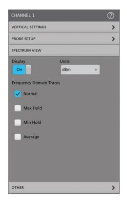
Spectrum View provides the ability to adjust the frequency domain using familiar center frequency, span and RBW controls.
