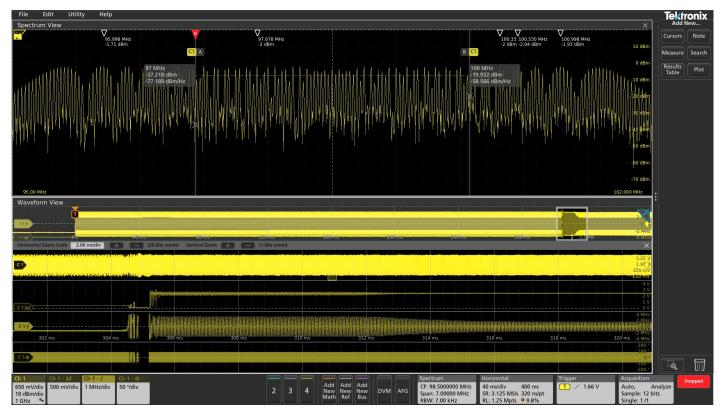
FIGURE 11. We've now zoomed in on the period of interest (roughly 300–320 ms after the trigger event). Notice that we can clearly see the amplitude fluctuating and the frequency changing over a broader range than it should be.
