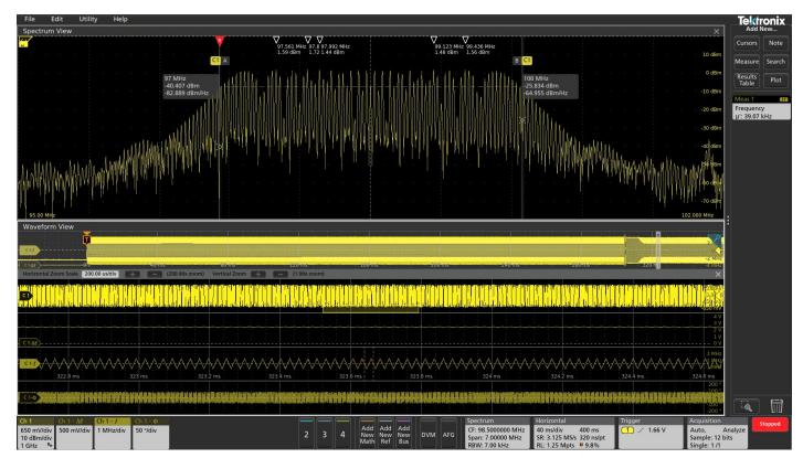
FIGURE 12. We've now zoomed in even further and can easily view the triangular frequency modulation in use and can confirm through the automatic measurement in the results bar that we are getting the correct modulation rate of 39.07 kHz.
