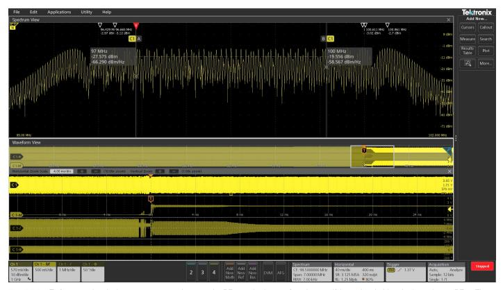
FIGURE 13. To focus on the clock turn-on, we can trigger on the RF magnitude waveform by specifying a threshold and edge using an RF vs Time Trigger setting. (Note: this measurement was made with more recent firmware than Figures 10–12.)
