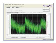
The ADS-B INTEGRITY™ software application, supports Supplemental Type Certification (STC) and post approval testing for ADS-B Out equipment installations. For accuracy and integrity performance test, the software controls the VIAVI IFR6000 or IFR6015 Transponder Test Set. An additional positional accuracy test is accomplished with the VIAVI GPSG-1000 Positional Simulator.
