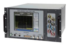
The RGS-2000NG TCAS Test Set is an RF signal generator/receiver for testing Traffic Alert and Collision Avoidance Systems (TCAS) with an option available for testing transponder LRUs. The RGS-2000NG was designed with modern software-driven digital modulation technology and is the RGS-2000 replacement for engineering development, design validation, manufacturing and return-to-service testing.
