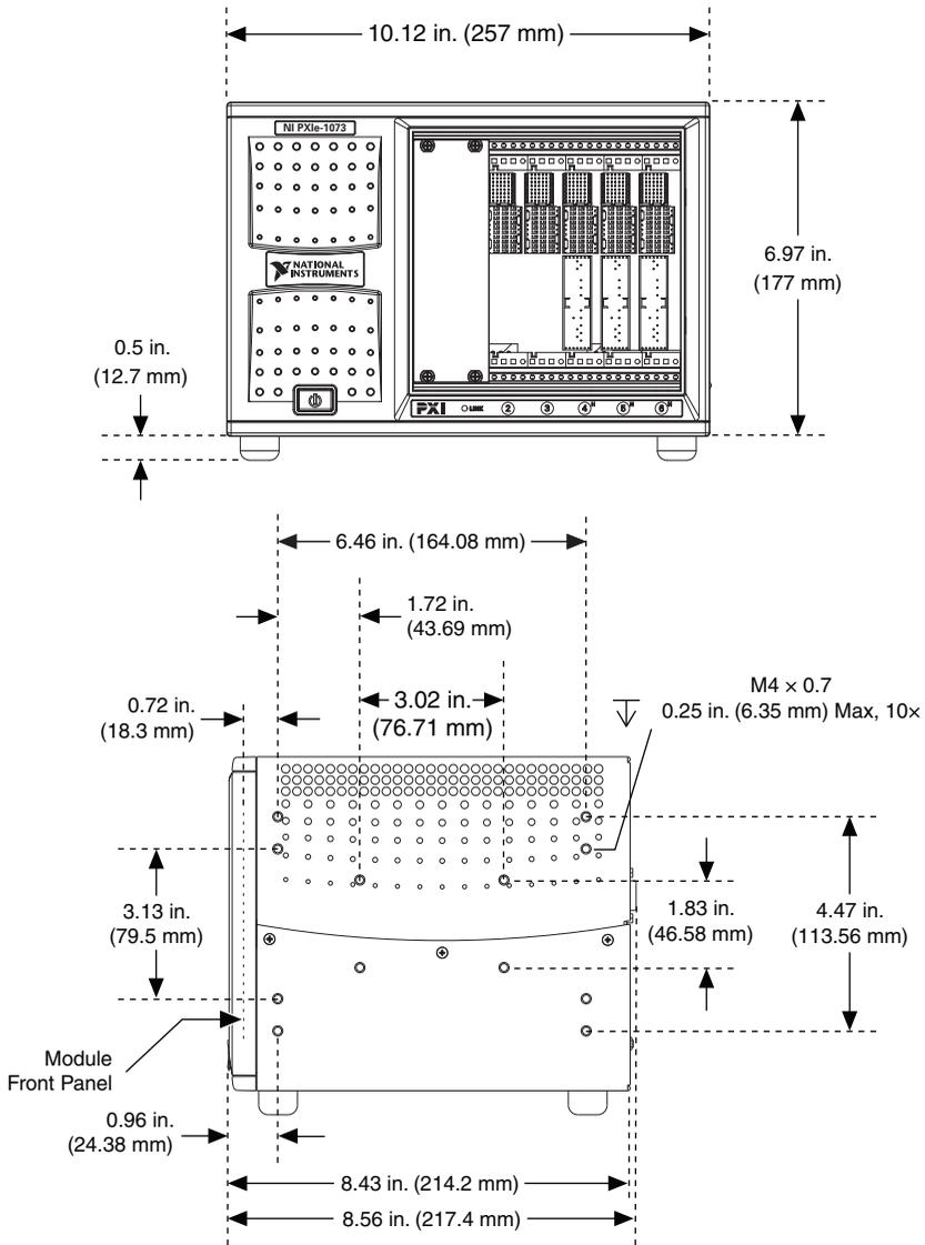
**Figure 4. PXIe-1073 Chassis Dimensions (Bottom)**
