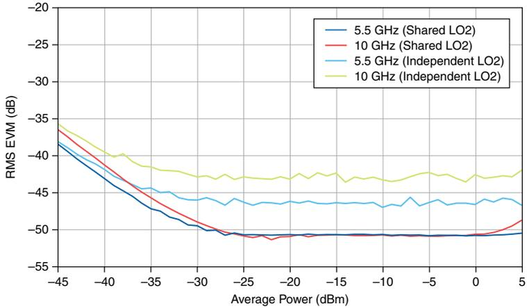
**Figure 16.** IF 5G NR 2 CC x 100 MHz RMS EVM versus Average Power, Measured<sup>14,16</sup>
