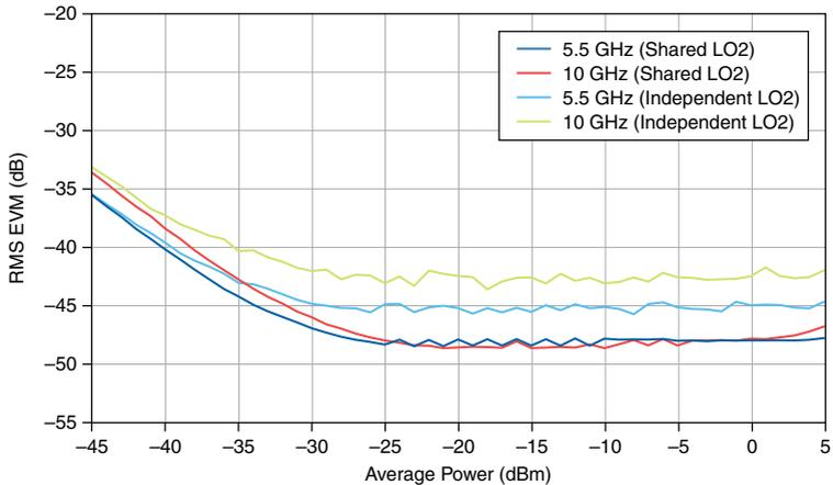
**Figure 17.** IF 5G NR 1 CC x 400 MHz RMS EVM versus Average Power, Measured<sup>14, 17</sup>
