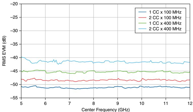
**Figure 20.** IF 5G NR RMS EVM versus Frequency (Independent LO2), Measured<sup>14, 19, 20</sup>
