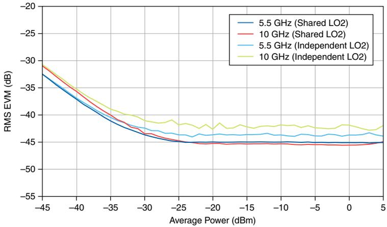
**Figure 18.** IF 5G NR 2 CC x 400 MHz RMS EVM versus Average Power, Measured<sup>14, 18</sup>
