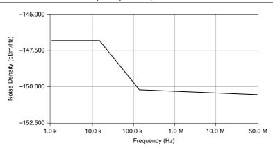
Figure 4. PXIe-5122 Spectral Noise Density, 0.2 V Input Range, Noise Filter Enabled,  $1~M\Omega$  Input Impedance, Nominal
