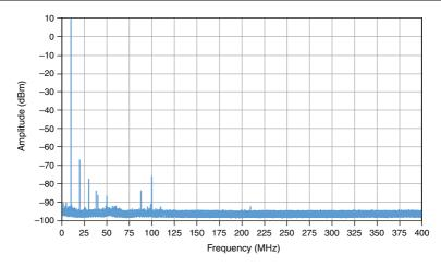
Figure 10. 9.5 MHz and 10.5 MHz Dual-Tone Spectrum<sup>23</sup>, Measured
