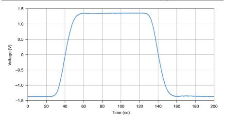
Figure 7. Square Waveform Step Response at 12  $V_{pk-pk}$ , Measured
