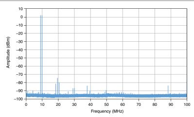
$<sup>^{22}</sup>$   $\,$  With the digital filter enabled and at -1 dBFS, 2  $V_{pk\text{-}pk},$  and 200 MS/s. Noise floor is limited by the noise floor of the measurement device.
