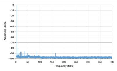
Figure 3. 10 MHz Spectrum<sup>13</sup> at 2 V<sub>pk-pk</sub>, Measured
