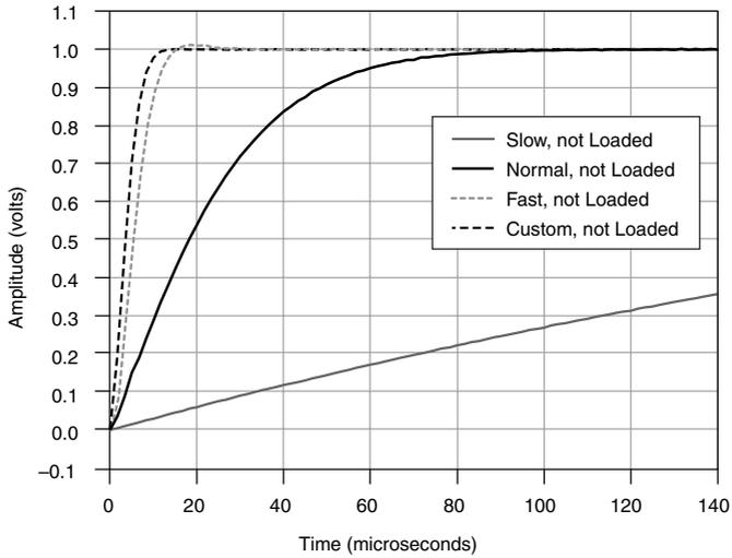
**Figure 4.** 1 mA Range, 100 nF Load Step Response, Typical
