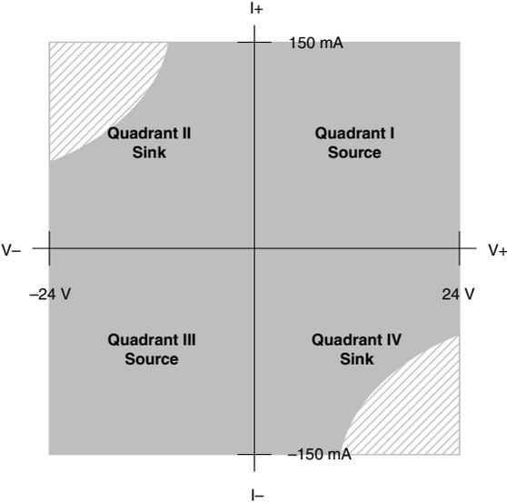
▨ Limit power sinking to 6 W per module.
