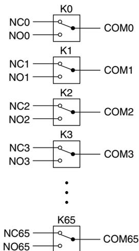
The following figure shows the PXI-2571 connector pinout.
