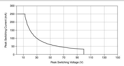
Figure 1. Peak Switching Voltage Versus Current
