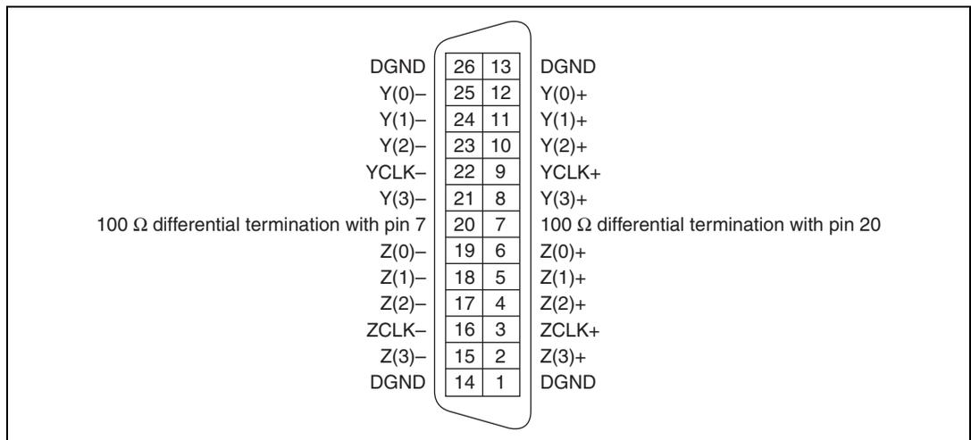
**Figure 3-3.** NI 1433 Medium/Full Configuration MDR Connector Pin Assignments**Table 3-2.** NI 1433 Medium/Full Configuration MDR Signal Descriptions
