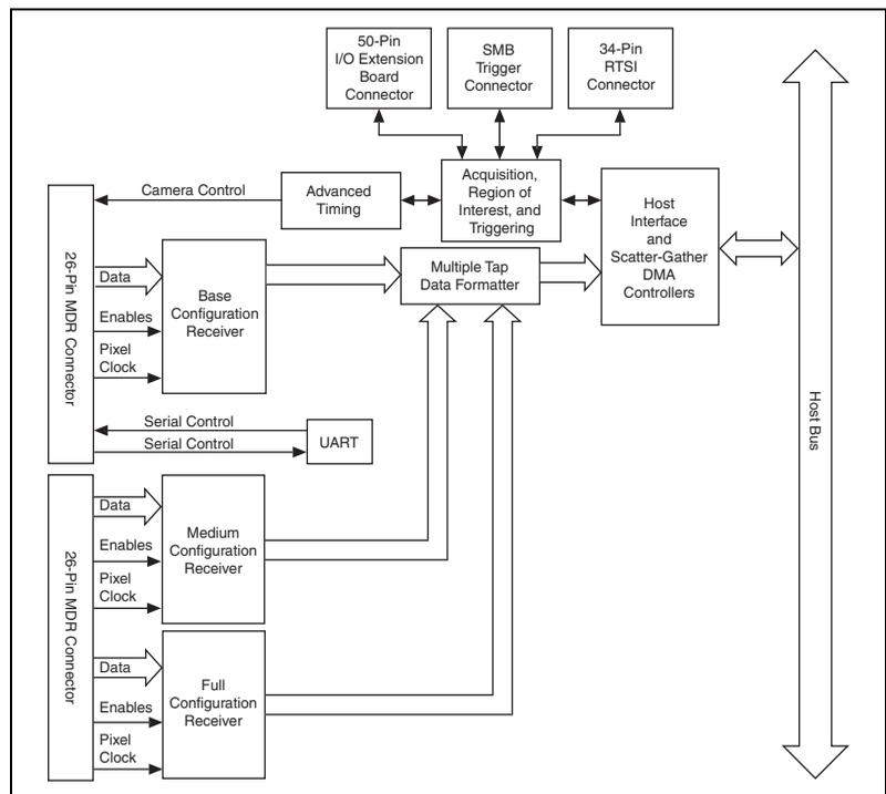
Figure 2-1. NI 1433 Block Diagram
