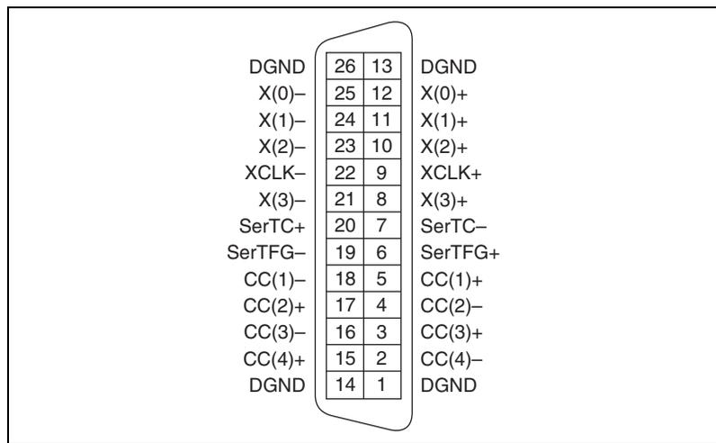
**Figure 3-2.** NI 1433 Base Configuration MDR Connector Pin Assignments
