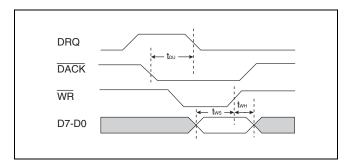
Figure 7. DMA Write
