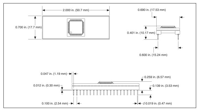
Figure 3. Mechanical Data 40-Pin Plastic DIP Package Compatible Module
