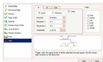
As well as the standard range of triggers found on all oscilloscopes, the PicoScope 6407 offers a comprehensive set of advanced triggers including pulse width, windowed and dropout triggers to help you capture the data you need.
