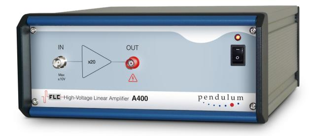
The Pendulum Instruments High Voltage Linear Amplifier A400 has a fixed amplification of 20 times and capable of bipolar high voltage output of ±200. Any other signal source with amplitude up to ±10 V can be used as an input device. The input amplitude should normally be kept within ±7.5 V. The A400 High Voltage Linear Amplifier is equipped with a microfuse rated at 15 mA, which will be blown if the input voltage exceeds 300% of the maximum.
