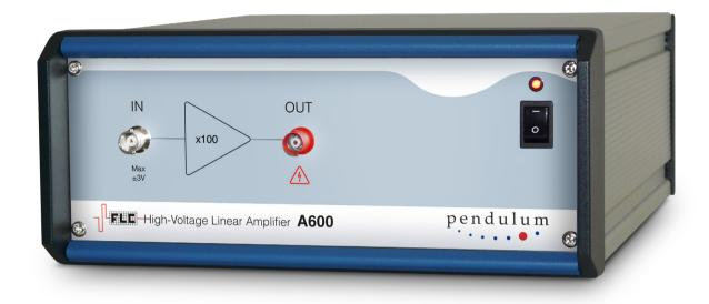
The Pendulum Instruments High Voltage Linear Amplifier A600 has a fixed amplification of 100 times and capable of bipolar high voltage output of  $\pm 300$ V. Any signal source with amplitude up to  $\pm 3$  V can be used as an input device. The input amplitude should normally be kept within  $\pm 3$  V. The A600 High Voltage Linear Amplifier is equipped with a microfuse rated at 15 mA, which will be blown if the input voltage exceeds 500% of the maximum.
