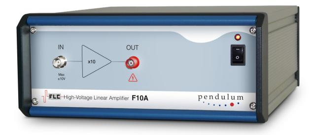
The Pendulum Instruments High Voltage Linear Amplifier F10A has a fixed amplification of 10 times and capable of bipolar high voltage output of  $\pm$ 100V. Any signal source with amplitude up to  $\pm$ 10V can be used as an input device. The input amplitude should normally be kept within  $\pm$ 10V. The F10A High Voltage Linear Amplifier is equipped with a microfuse rated at 15 mA, which will be blown if the input voltage exceeds 300% of the maximum.
