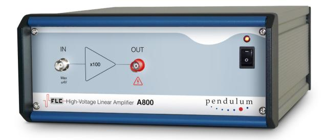
The Pendulum Instruments High Voltage Linear Amplifier A800 has a fixed amplification of 100 times and capable of bipolar high voltage output of  $\pm$ 400V. Any signal source with amplitude up to  $\pm$ 4 V can be used as an input device. The input amplitude should normally be kept within  $\pm$ 4 V. The A800 High Voltage Linear Amplifier is equipped with a microfuse rated at 15 mA, which will be blown if the input voltage exceeds 500% of the maximum.
