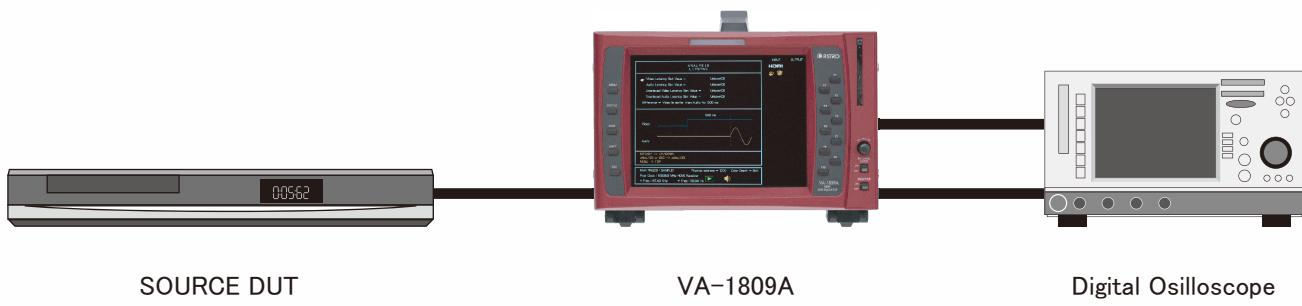
With using our HDMI protocol analyzer (VA-1809A), you can measure and also can display the amount of delay of image output signal and audio output signal from a SOURCE device. By connecting a digital oscilloscope, you can also measure the data by using video and audio trigger output from I<sup>2</sup>S output (TTL 3.3V) of VA-1809A.
