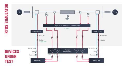
Typically, detailed models of the instrument transformers (CT, PT and CVTs) are used to provide signals to digital to analogue (D/A) converters.
