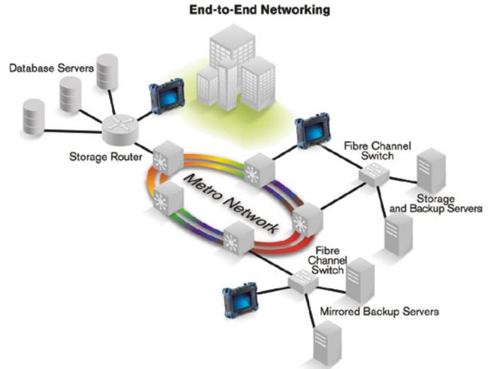
*Thanks to end-to-end network testing capabilities, EXFO's FTB-700G Series enables fast deployment and configuration of Fibre Channel networks. Communication between the transport network, interconnection devices and end nodes can be validated with features such as BER testing, latency measurement, buffer-to-buffer credit estimation and port login capabilities.*
