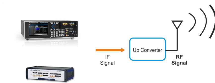
Figure 7: AWG for IF signals (TX) : Arb Rider AWG-4022 and AT-AWG-GS
