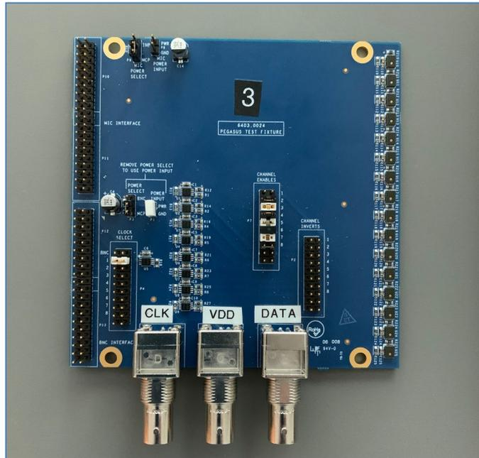
Figure 3. The PDM 16 test fixture with 16-microphone array.
