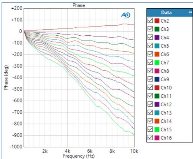
Figure 14. Phase response of the microphones in the array relative to Channel 1 (the 2nd closest mic to the speaker).
