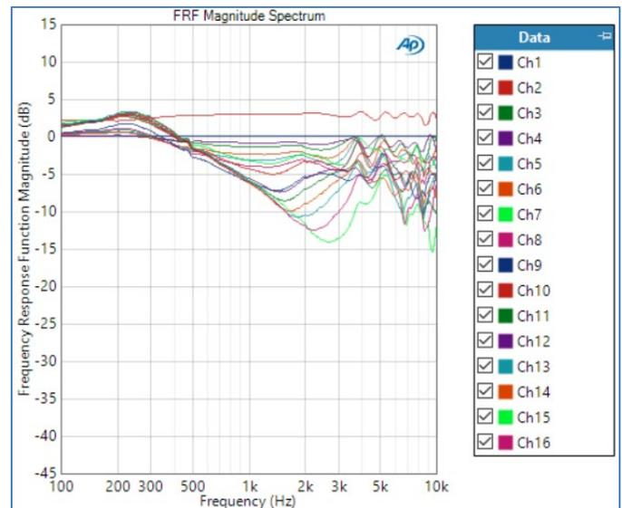
Figure 15. Transfer function magnitude between all DUT microphones and Ch1 microphone (at Test Point).
