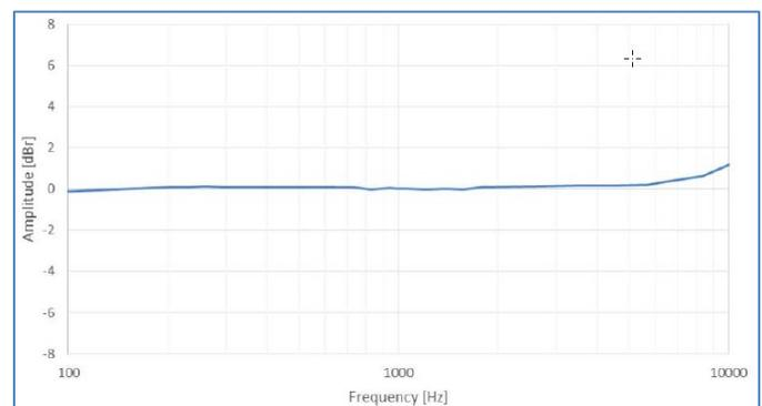
Figure 10. Manufacturer-specified typical frequency response relative to 1 kHz for the microphones in the array.
