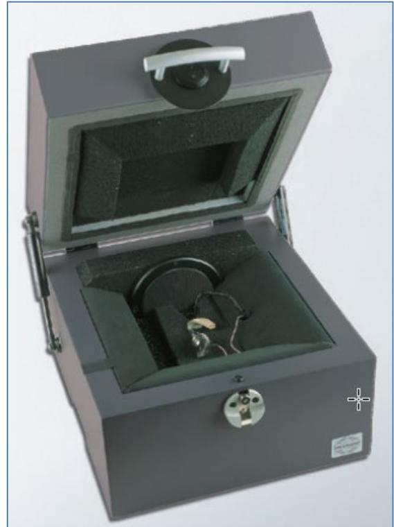
Figure 4. Interacoustics TBS25 sound test chamber.
