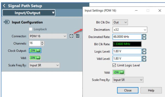
Figure 8. PDM 16 configuration settings used.
