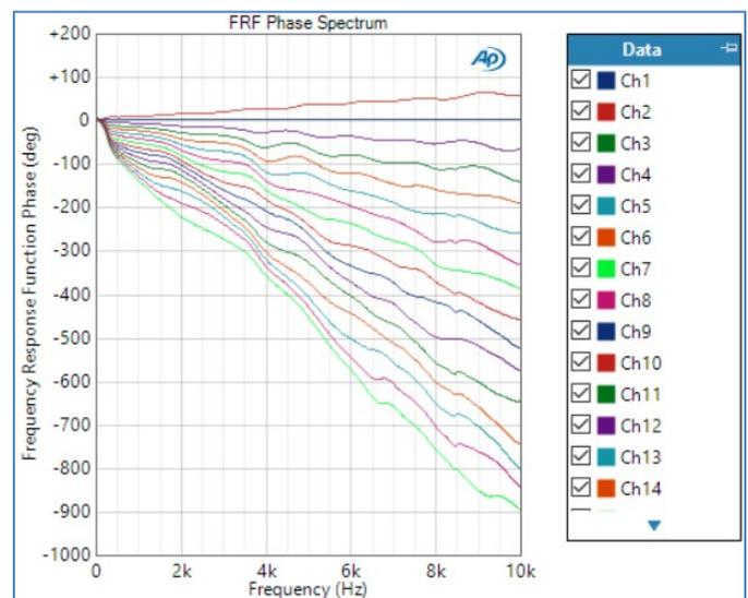
Figure 16. Transfer function phase between all DUT microphones and Ch1 microphone (at Test Point).
