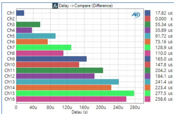
Figure 12. Delay of each microphone in the array relative to microphone position 1 (Ch2), as measured with Acoustic Response.
