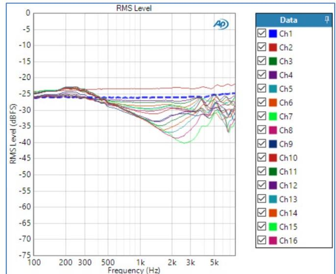
Figure 9. Frequency response magnitude of the 16 PDM microphones in the microphone array.
