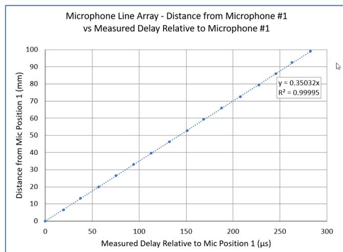
Figure 13. The delay measurements from Figure 12 plotted versus microphone position.
