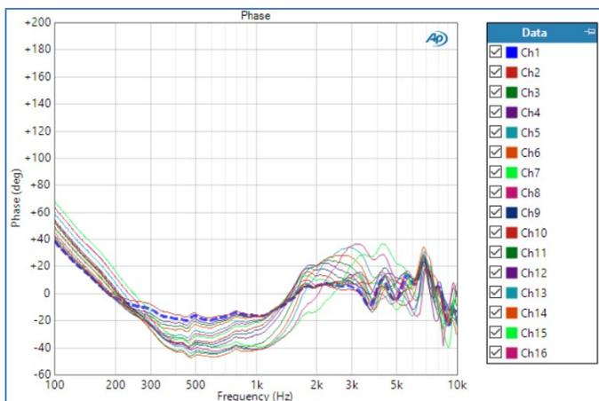
Figure 11. Phase response (input-to-output excess) of the 16 PDM microphones in the microphone array.
