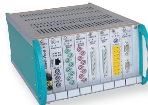
ADwin-Pro II-light , 7 module slots
