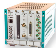
ADwin-Pro II-mini , 5 module slots
