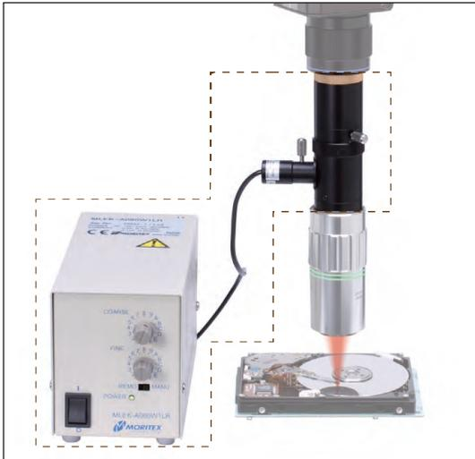
The LV-0185 is an option which illuminates a target coaxially with laser beams. The White LED and the laser beam illuminate the detecting part in the same working distance, and sharpens the images of the LV-0181. Mounting an objective lens is more effective to focus the light. It facilitates laser irradiation to a minute detecting part and a rear side where light is difficult to be illuminated.
