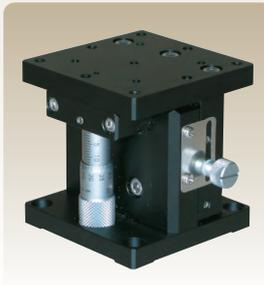
The Z stage enables precise alignment of the sensor up/down position. Using it together with the LV-0030 magnet stand, focusing of laser beams and image, and fine adjustment in horizontal direction can be performed.
