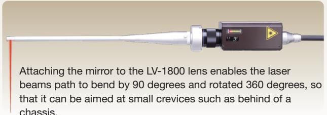
Attaching the mirror to the LV-1800 lens enables the laser beams path to bend by 90 degrees and rotated 360 degrees, so that it can be aimed at small crevices such as behind of a chassis.
