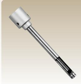
Attaching the mirror to the LV-0301, it enables the laser beams path to bend by 90 degrees, so that it can be aimed at narrower space.
