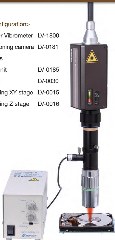
Installing the LV-0181 (Built-in positioning camera), the LV-0185 (Illumination unit) and an objective lense to the LV-1800 enables micro spotting of laser beams and image observation by epi-illumination. It makes laser positioning to microstructures and detection of multipoint parts possible.
