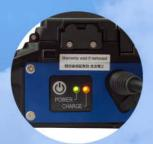
Charge the battery in the splicer while working
