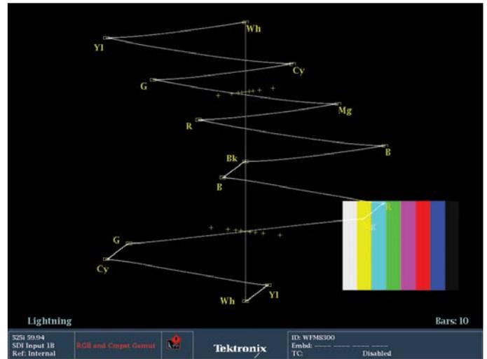
Figure 43. P'b delayed timing error on Lightning display.
