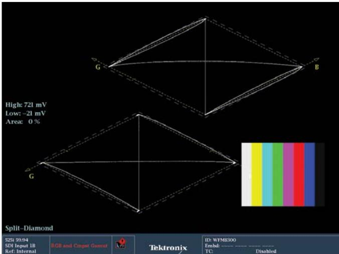
Figure 16. P'b timing error shown on Diamond display.
