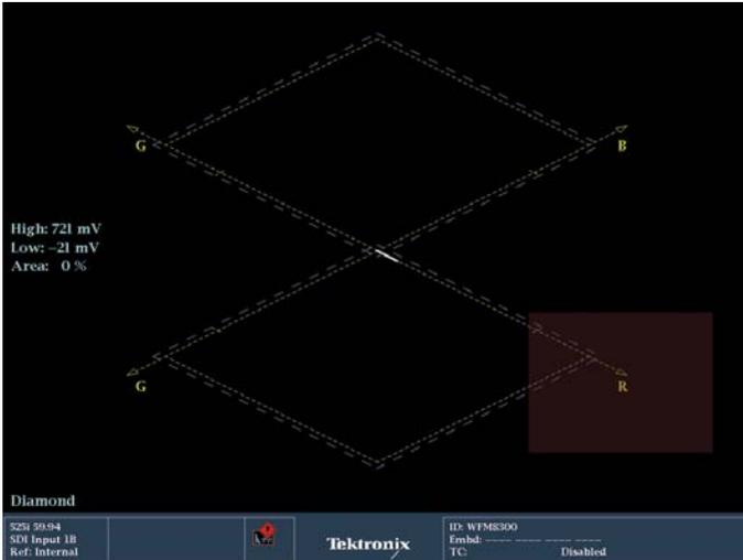
Figure 17. Red balance error on Diamond display.
