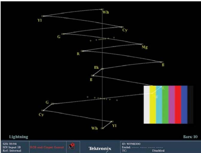
Figure 42. P'b advanced timing error on Lightning display.
