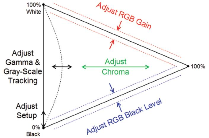
Figure 25. Using the Spearhead display for color correction.
