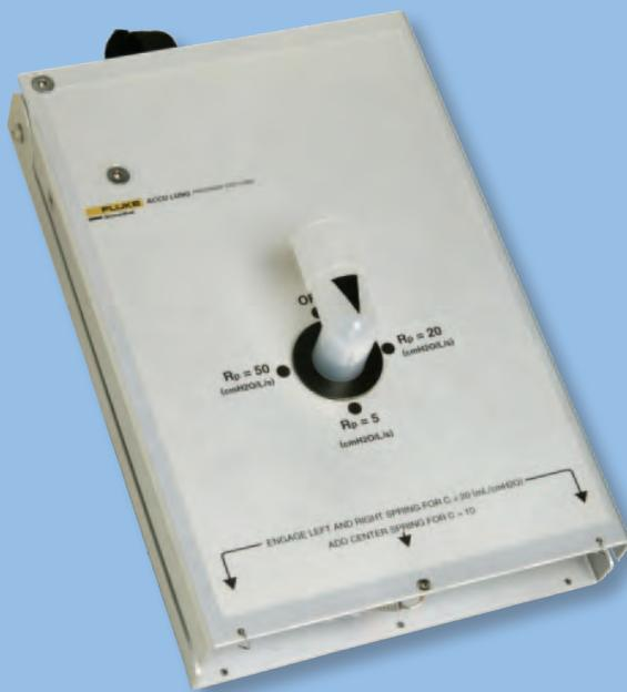
The ACCU LUNG Precision Test Lung is a lung simulator that presents a specific load comprised of user-selectable compliance and resistance for the purpose of evaluating ventilator performance according to clinical expectation and manufacturers' specification. It is a portable unit that can be hung from a cart, the ventilator itself, or hand-held, thus presenting a zero footprint.
